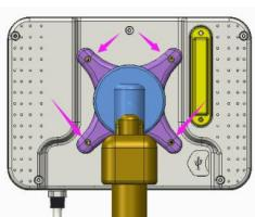
On the back of the product, 4 M4 75\*75mm thread holes are reserved, and the hole position of the bracket (refer to the left) is aligned with the thread hole, and the screw is screwed into the M4 specification.
