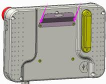
Through sketch left hanging structure, specifications of the screws fixed in the shell reserved above two holes, can suspended in a desired position control.
