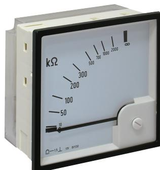
The indicating device EH 5861 is externally connected to the insulation monitor on terminals UA / GA (0 - 10 V) and shows the actual insulation resistance of the voltage system to ground.
