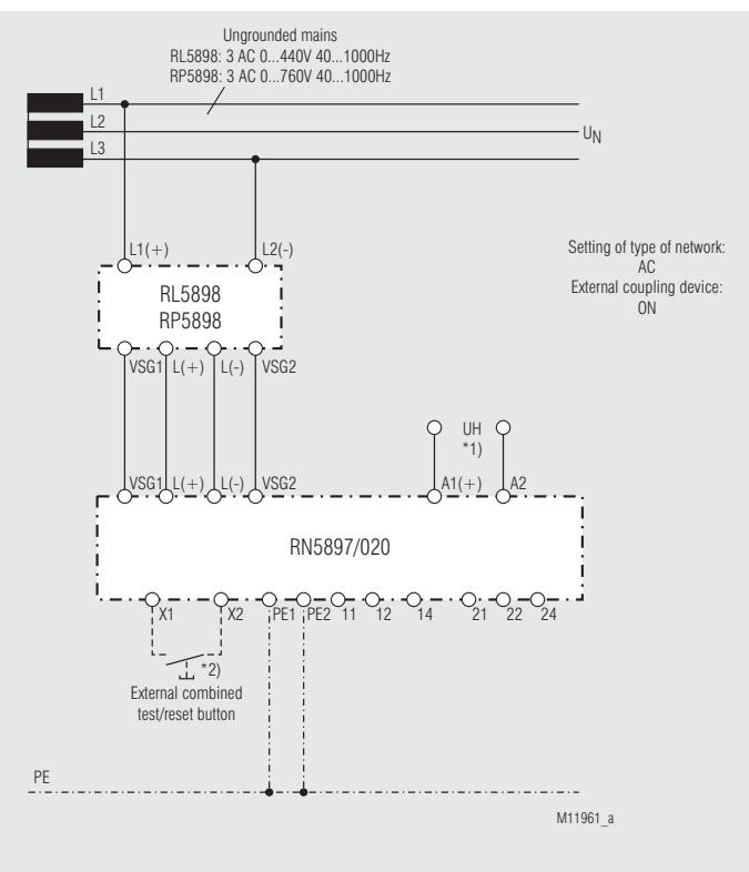
\*1) Auxiliary voltage  $U_H$  (A1(+)/A2) can also be sourced from the monitored voltage system.
