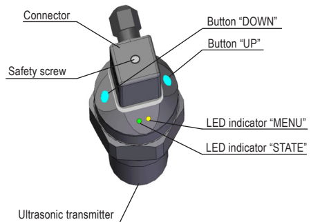
Fig. 17: Full view of ultrasonic level meter
