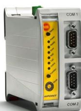
The software-based RS interface is configurable to RS232 or RS485. In this way, up to two control systems can be connected simultaneously between which one can switch to online mode during remote maintenance.
