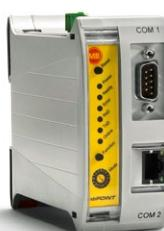
All mbPOINT devices with an ETHERNET or Wi-Fi interface possess a so-called router functionality. Remote data transmission clients can dial in via an integrated PPP server and access the remote network. According to the set operating mode, a further control system can be connected to the serial interface which can also receive remote maintenance.
