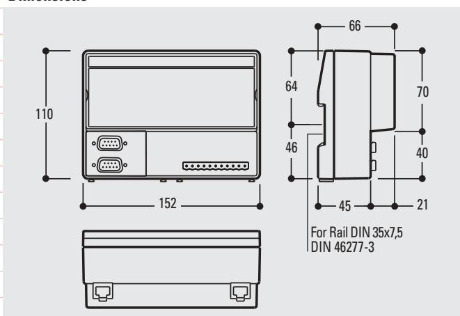
The Control Unit offers a high degree of flexibility. It can function as a slave device on a Modbus RTU, Modbus TCP, CANopen, Profibus network, and act as CANopen master on the underlying CANopen system (I/O modules and third party devices). Thus the Control Unit is the ideal device for modular systems with distributed control architecture. With integrated industry standard open communications, the Control Unit makes it possible to easily communicate with decentralized I/O nodes or other PLCs.
