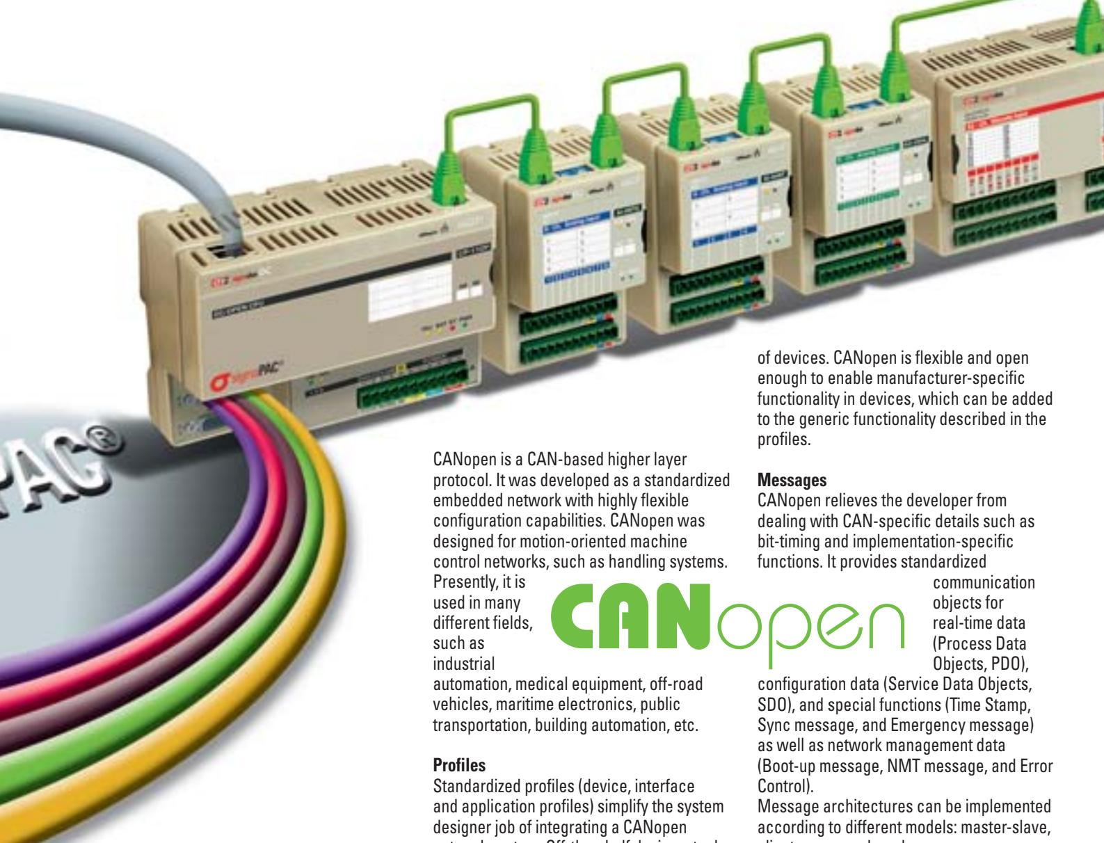
CANopen is a CAN-based higher layer protocol. It was developed as a standardized embedded network with highly flexible configuration capabilities. CANopen was designed for motion-oriented machine control networks, such as handling systems. Presently, it is used in many different fields, such as industrial automation, medical equipment, off-road vehicles, maritime electronics, public transportation, building automation, etc.
