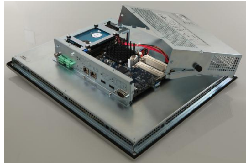
Integrated UPS with battery pack (rear of the system mounting)
