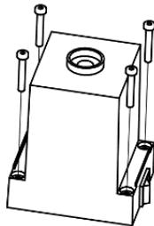
Fastening with screw (supplied with the lamp)
